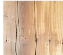
Cracks are the result of the movement of wood fibers during the drying process or due to the fall of the tree. Once stable, the cracks do not tend to open more significantly. Yet these tops are locked with a flat bar on their undersides.
